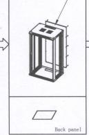
(3) Fixed the back panel on the frame with M5.5 \* 10 self-tapping screw
