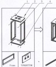
(1) Assembling the Top&Bottom and frame with M5.5 \* 10 self-tapping screw Mounting profile
